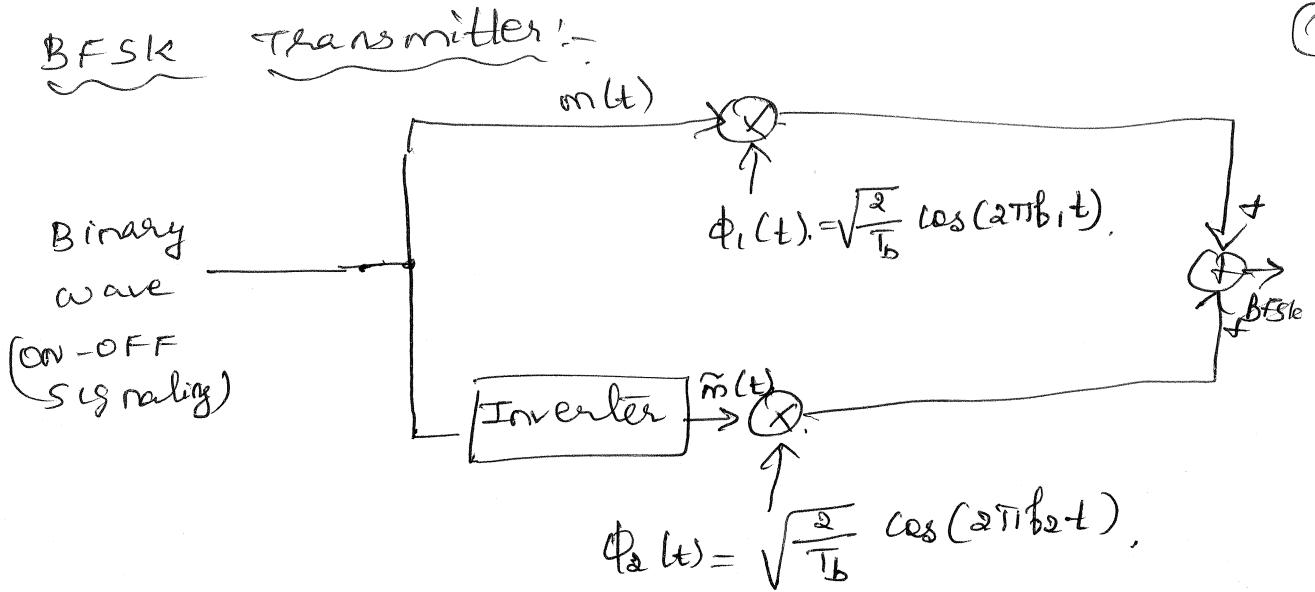
The input binary sequence is represented in its ON-OFF form.
