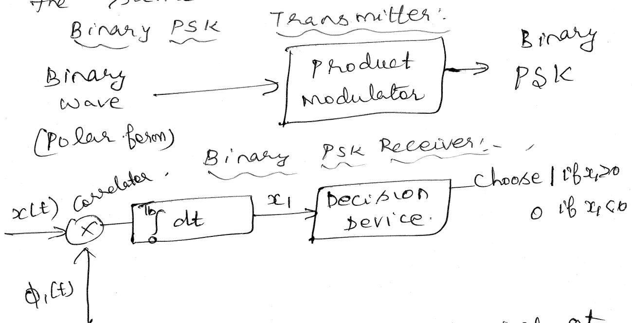
The noisy PSK signal received at the channel output is given to a correlator. The locally generated coherent reference signal  $\phi_r(t)$  is also applied to the correlator. The correlator produces a scalar  $x_1$  and is compared with a threshold of '0' volts.
