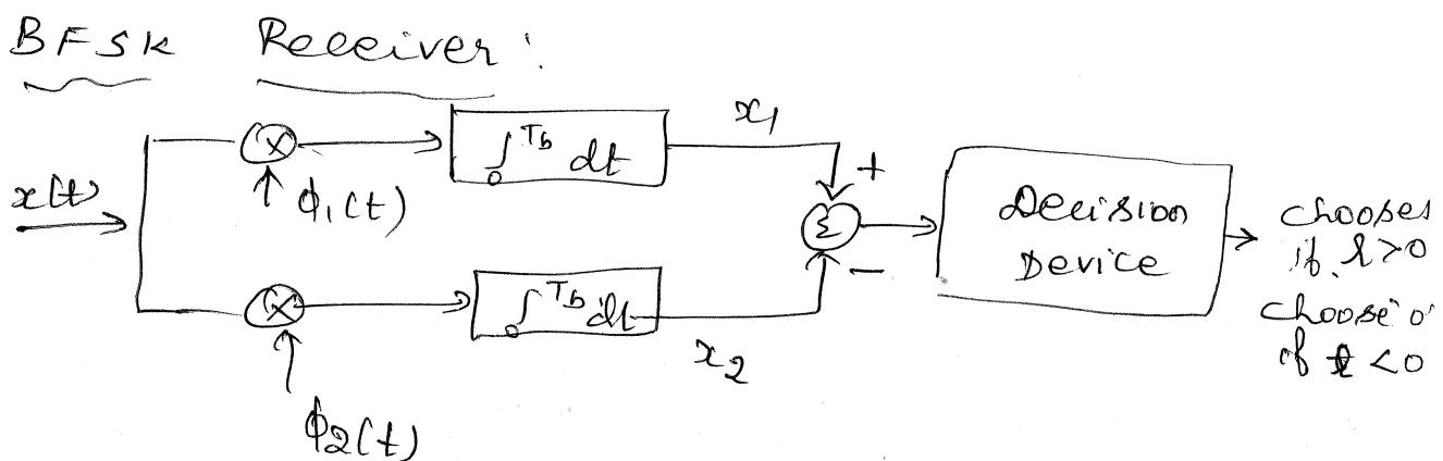
The noisy received wave  $x(t)$ , is given as an i/p to the receiver. Receiver consists of two correlators with a common input which are supplied with locally generated coherent reference signals  $\phi_1(t)$  and  $\phi_2(t)$ . The correlator outputs
