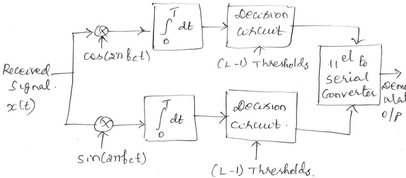
The noisy received signal is given as an i/p to the receiver. Received signals are passed thro' the multiplier and to produce 'L' level signals. In integrator, the decision circuit compares L-level signals against  $(L-1)$  decision thresholds. The two binary sequences so detected are then combined using parallel to serial converter to reproduce the original binary sequence.
